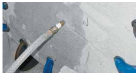
WATER INTRODUCED THROUGH CAST-IN NOZZLE
