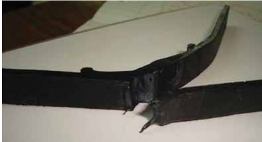
TESTED COUPON WITH PEEL FAILURE OF THE WELD
