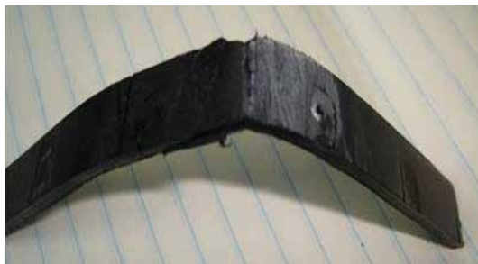
TESTED COUPON WITH PEEL FAILURE OF THE WELD
