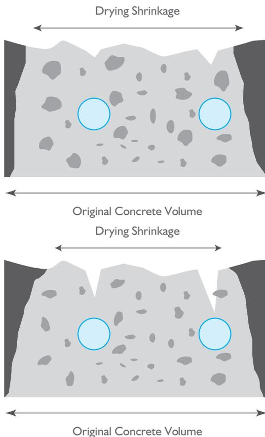
A greater volume of stiff aggregate reduces concrete shrinkage, as the aggregate provides restraints. This reduces the tensile stresses and thereby minimises concrete cracking.
