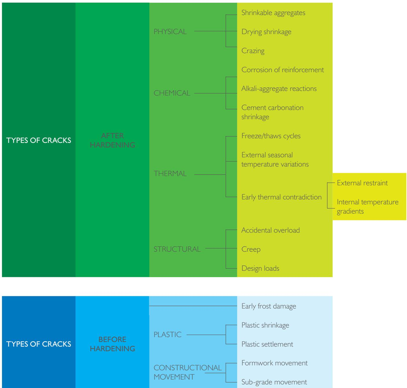
Figure 1: Types of cracks and their causes
